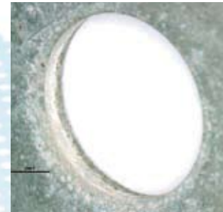
16 months 10% red rust - 70% white rust
